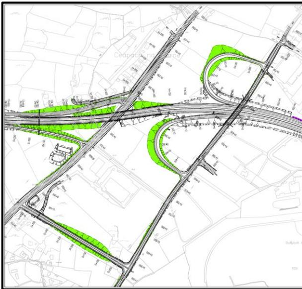
The refined N17 Junction comprises a grade separated junction and associated link roads. The slip termini, as well as all junctions integral to the operation of the junction, are signalised.
